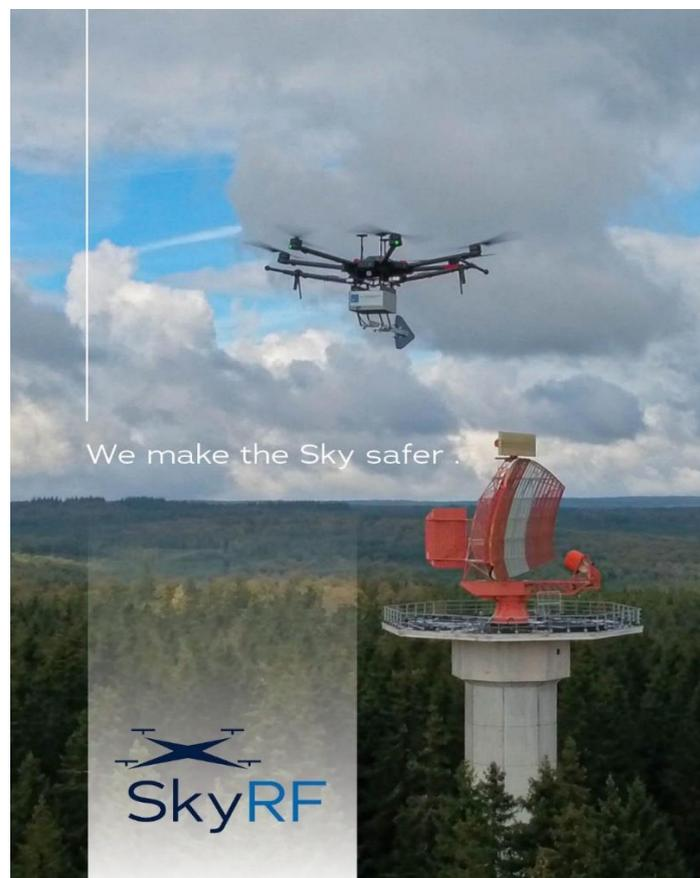
*SkyRF performing drone measurements on a collocated PSR-SSR*
